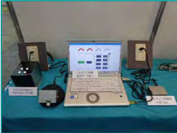
C01. Socionext Introduction about 4 th Gen LSI. Capturing the information by radio-freq human sensed sensor, and displaying it on PC screen through PLC transmission.
